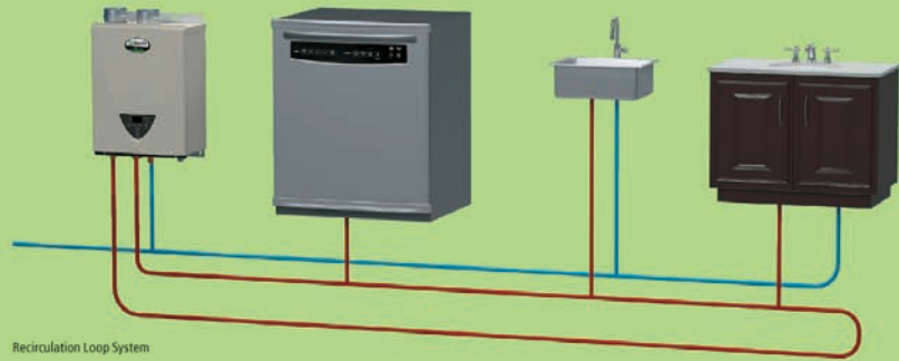
Recirculation Loop System
