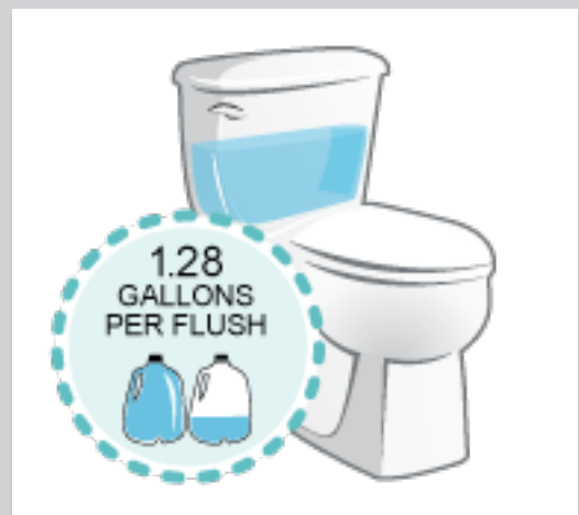
High efficiency toilets (HET) use 1.28 gallons per flush.
