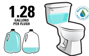
High efficiency toilets (HET) use 1.28 gallons per flush.
